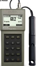
HI 98186 portable Dissolved Oxygen Meter has extended ranges of up to 50 ppm or 600% saturation. This instrument includes barometric pressure measurement and calibration with a user selectable unit (mmHq, atm, mbar, psi, kPa) as well as a 1 or 2 point temperature calibration. Salinity, pressure and temperature compensations enhance the precision of your readings.
