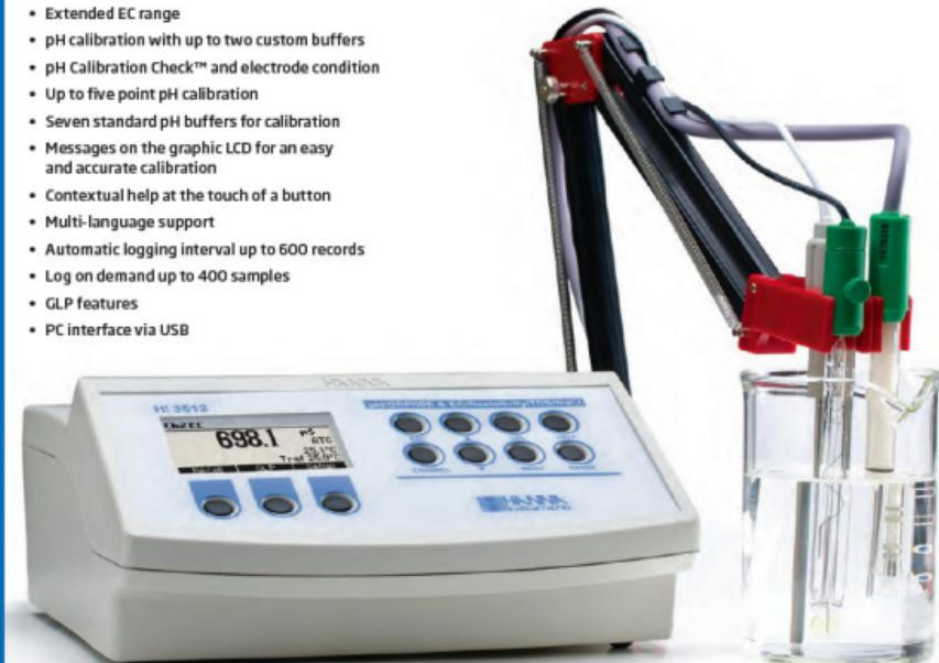
The HI 3512 is a multiparameter, 2 channel professional benchtop meter with a graphic LCD, designed to provide accurate laboratory results. Channel 1 features pH/ORP/ISE and temperature measurement capability while channel 2 measures EC/TDS/NaCl/ Resistivity and temperature.
