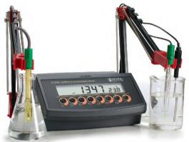
HI 2550 is a multiparameter 2 channel instrument that measures up to 7 parameters. With this single laboratory bench meter you can measure pH, ORP, ISE, conductivity (EC), TDS, NaCl percentage and temperature.
