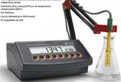
HI 2300 measures EC, TDS, NaCl and temperature. In conductivity and TDS ranges (up to 500 mS/cm and 400 g/L respectively) the instrument automatically chooses the best scale to maintain the highest accuracy.
