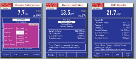
the HI 4222 and HI 4522, the meter calculates the sample concentration automatically and then logs it into an ISE methods report. 200 reports can be saved for future recall. The entire process can be repeated on multiple samples without reentering sets of parameters.
